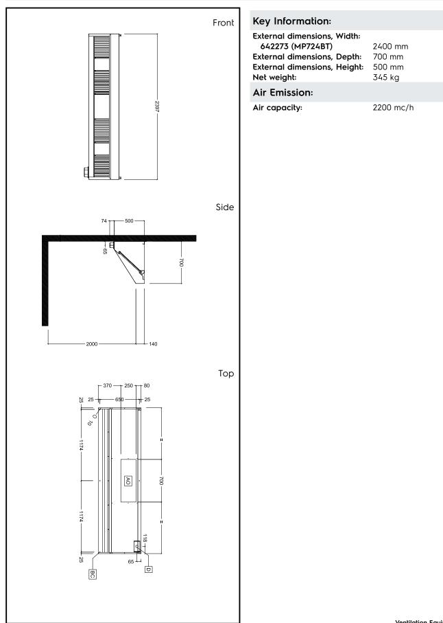
Ventilation Equipment 430 S/S Wall Hood+Filters 2400X700mm
